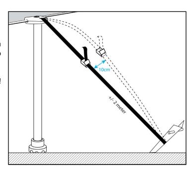
You can also put extra side clamps in the line of the welded seams. It is in any case always a good idea to put the clamps at the end of the welded seams, it will give you less 'wrinkles'.
