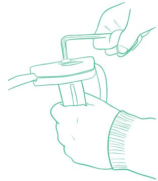
If everything has been assembled correctly, the assembly will fit perfectly in the pre-drilled 16 mm hole (see step 5).
