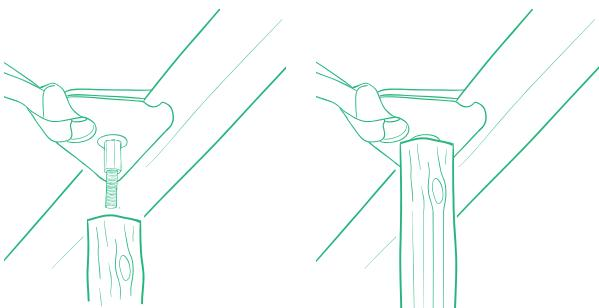
When all the poles are attached, raise them up one by one under the stretch tent and fit a pole foot to every aluminium pole. You may also tighten the tension straps slightly, but not yet to full tension.
