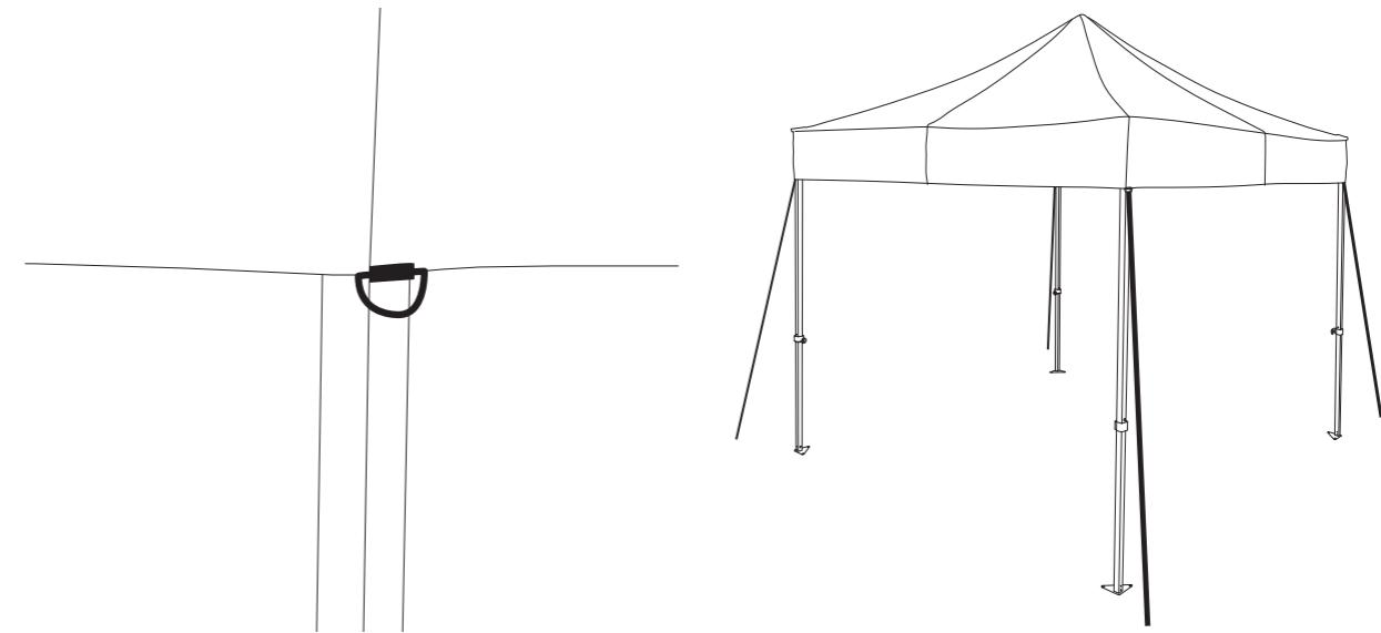
You can secure the bottom edges of the side walls using tent pegs in the loops provided for this purpose. There are also holes in the base plates of the legs for this purpose. You can also place weights on the base plates.
